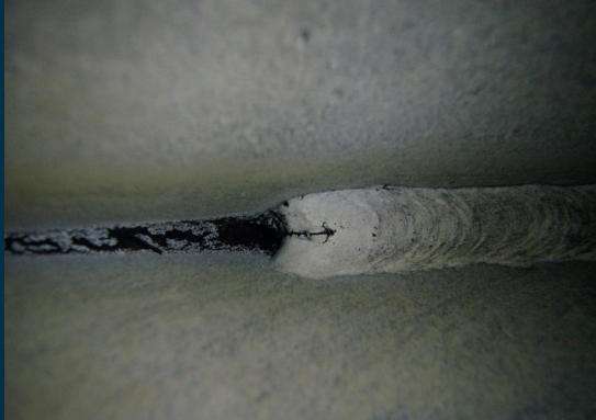
Black on white visible magnetic particle testing
